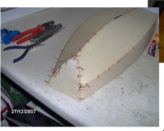
By the 27th Dec I had the Hull skins stitched together with copper wire, as per full size construction; all ready for the glassfibre tape and resin
